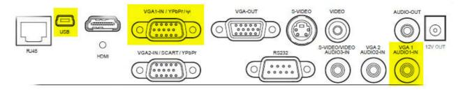
Connect from the PC's External VGA output to EX615 VGA1 In
